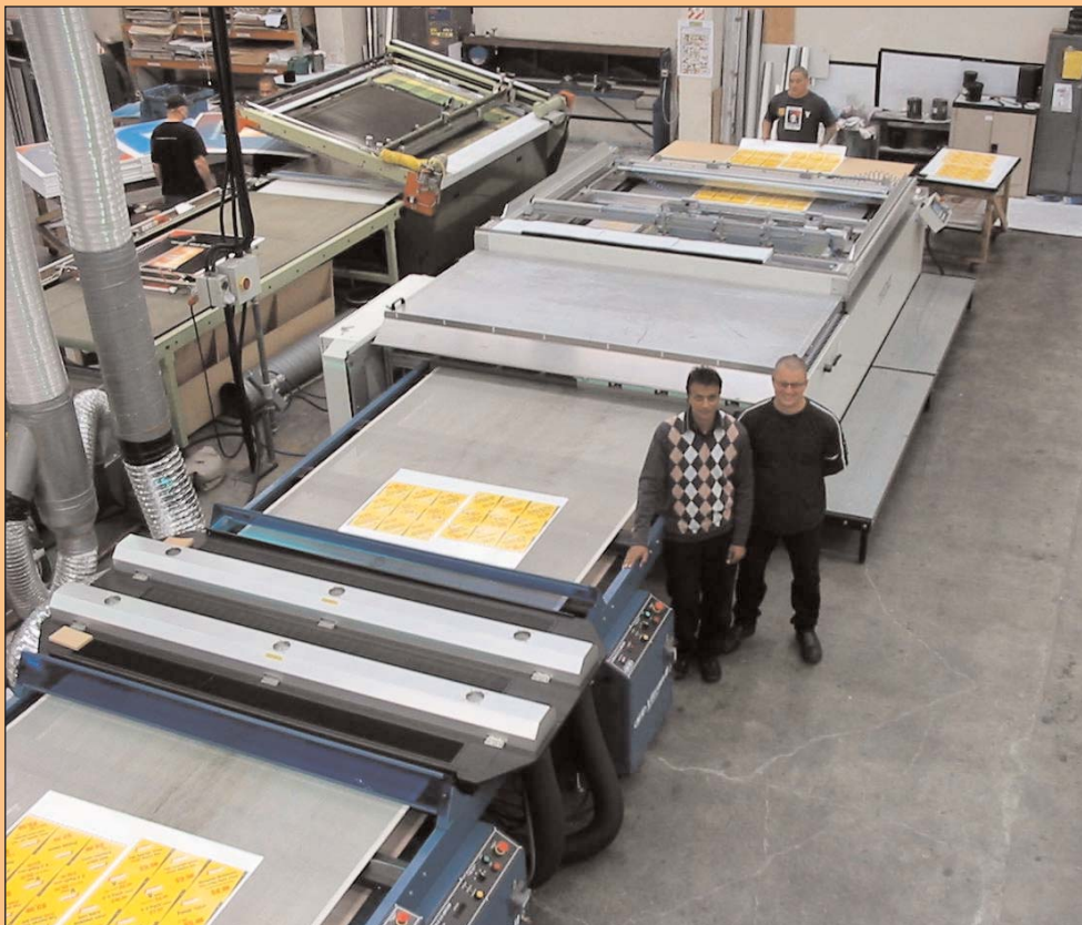
Leading Wellington screen print company, MESH Ltd, is already counting the benefits of its recent installation of a Thieme 5050 printer and a Vitran UV curing system.
